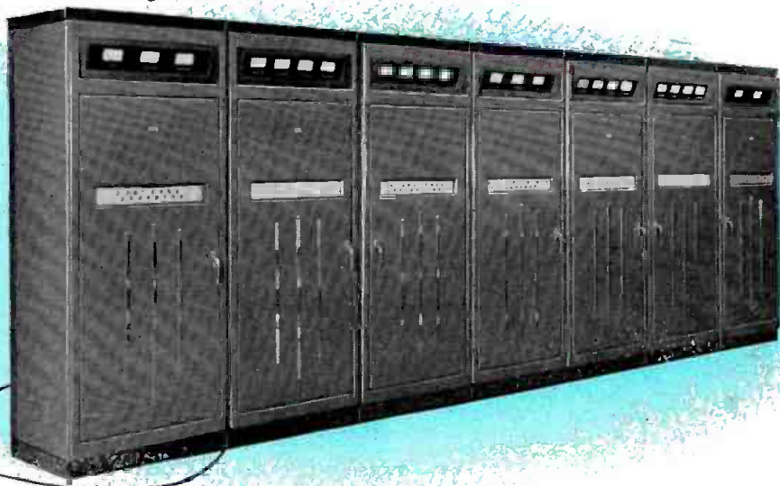
SERIES 9000 (LOW BAND) 25 KW VHF TELEVISION TRANSMITTER
